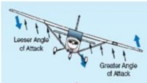
If a wing with dihedral encounters a disturbance in roll it will also sideslip which presents the lower wing to the airflow at a greater angle of attack. This means that the lower wing creates more lift and has the tendency to roll back to the wings level position.
