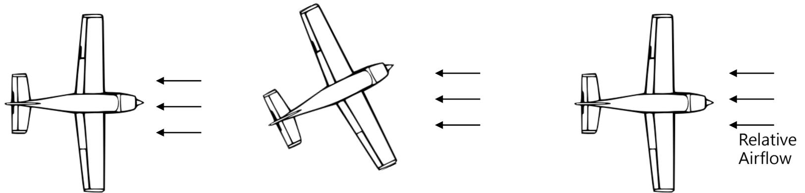
If the aircraft is disturbed (uninvited yaw) the fin is presented to the airflow at a different angle of attack which has the tendency of returning the aircraft to its original starting position.
