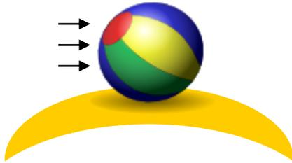
If we imagine a ball at the top of a hill... If the ball is pushed sideways, it will continue to depart from its original position as it rolls down the hill
