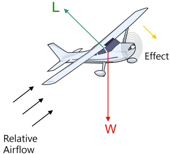
Aircraft which have a high keel (high fin, T-tail etc) and a low centre of gravity will mean that there is a restoring force after a disturbance in roll.
