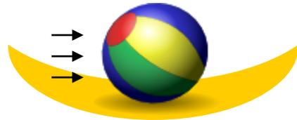
If we imagine the same ball at the bottom of a concave slope.. If the ball is pushed sideways it will eventually return to its starting point
