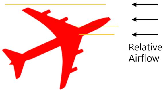
Sweepback works by the lower wing after the sideslip creating more lift than the upper wing because the lower wing has a greater area presented to the airflow. This will tend to return the aircraft to the wings-level position
