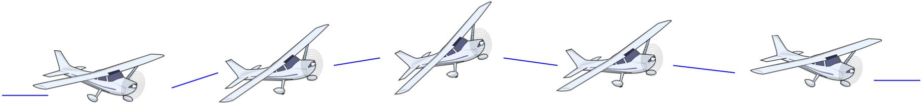
The aircraft above shows POSITIVE dynamic stability it returned to its starting point with minimal oscillations.
