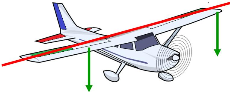
Pulling the control column rearwards causes the aircraft to pitch up relative to the lateral axis.
