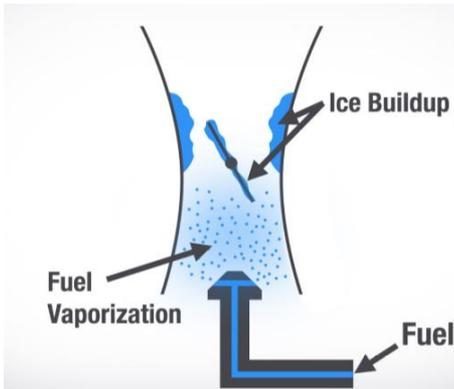
As air moves towards the engine, it speeds up. This is because the pathway includes a venturi (where there is a narrowing of the pipe).
