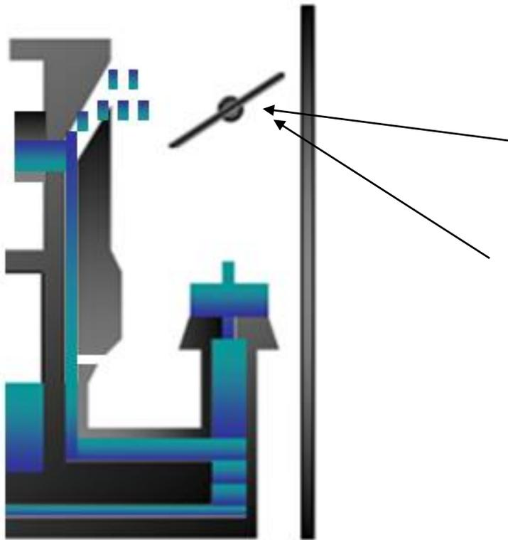
When the pilot pushes the throttle in (opening the throttle) – the butterfly moves towards the position where the maximum air can flow past. The more air entering the engine the more power is produced.
