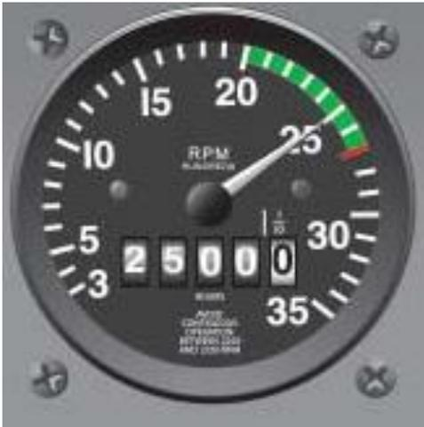
The throttle setting can be seen on the rpm gauge. The red line indicates the maximum rpm allowable. Every engine will have a maximum time that it can run at maximum rpm and also a maximum duration over the maximum rpm (this is not long!)
