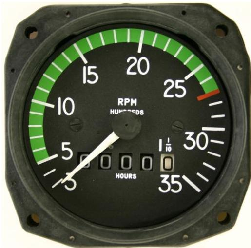
The simplest way to lean the mixture is to use the rpm gauge. The pilot should note the rpm and then slowly pull out (twist if in a C152) the mixture control until a small rpm drop is observed.
