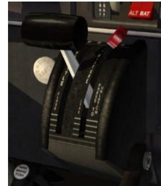
If you are flying in a PA28 aircraft the mixture is the lever next to the throttle. It is red and shaped differently from the throttle to help minimise confusion between the two levers.
