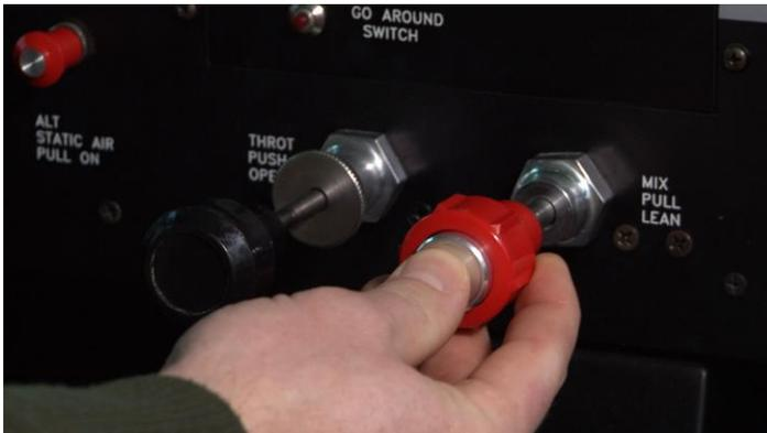
If you are flying in a Cessna aircraft, there are two ways of moving the mixture control – one is by using the “override” knob which allows the knob to be moved like a throttle. For finer adjustments, the mixture control can be twisted in and out.
