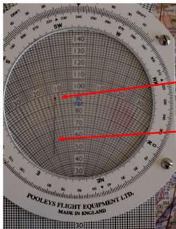
Rotate bezel until the desired track lies under the "true heading" mark
