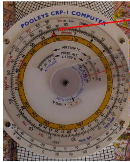
On the calculation side of the flight computer, set the ground speed under the "per hour" index
