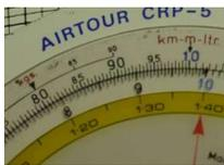
88 kts on **inner** (RAS) scale reads 90 kts on the **outer** (TAS) scale
