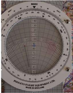
Rotate the bezel until your vertical line is parallel with the slanted lines on the wind computer face
