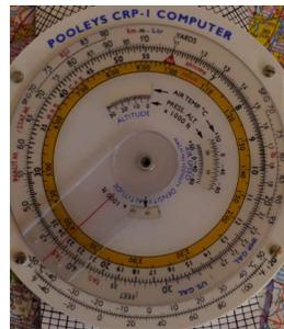
If your groundspeed is over 100 kts – just take off a zero – the flight computer doesn't have a decimal point
