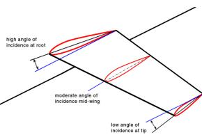
The "twist" of the wing ensures that the outer section of the wing has a lower angle of attack than the inner portion
