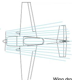
Thrust from the propeller accelerates the airflow and adds kinetic energy to it
