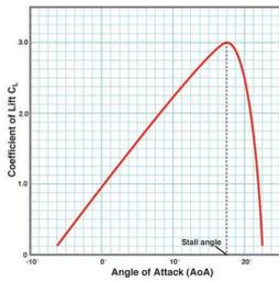
Stalling of the wing occurs above the stall angle or "critical angle" of attack
