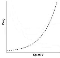
Parasite Drag is caused by the aircraft being in the airflow
