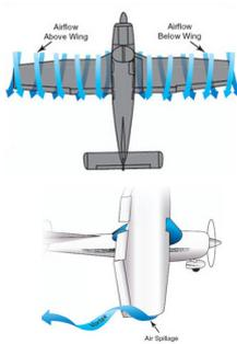
Lift is created by the pressure differential between the upper and lower surfaces of the wing
