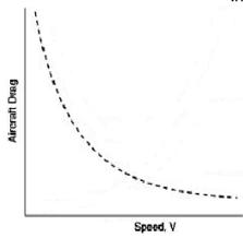
Induced drag is caused by the generation of lift
