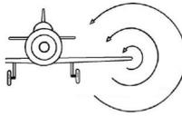
The downward pressure on the wing causes drag as does the vortices which are created behind the wing
