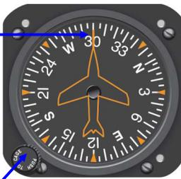
Setting knob (releases gyro so that compass card can be rotated)
