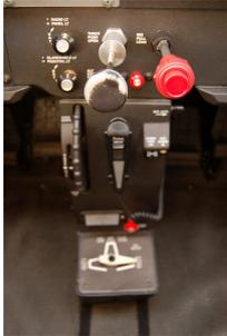
It is safer to shut down an engine using the mixture control at "idle cut off"
