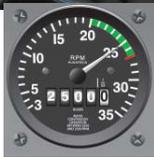
ALWAYS use CARB HEAT selected to ON / HOT when using throttle settings below the GREEN ARC on the RPM gauge
