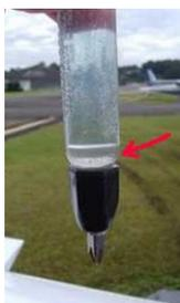
Before flight all drain points on the aircraft should be inspected for fuel contamination
