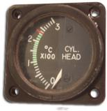
Some aircraft have Cylinder Head Temperature (CHT) gauges to monitor engine heat build up
