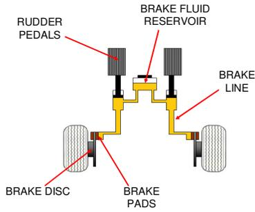
The brakes on the rudder pedals push an actuator
