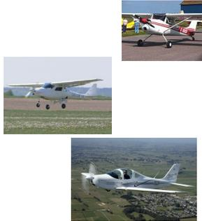
Generally 3 wheels – 2 mains and either a tailwheel or nosewheel
